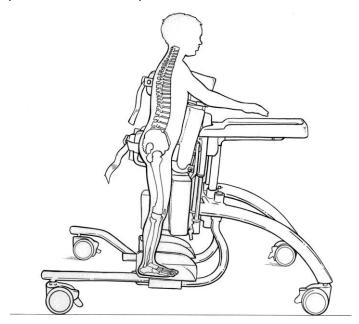
The footplates are adjustable to facilitate a standing base as wide as or slightly wider than the pelvis.
