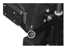
The width between the pelvic supports can be adjusted. Loosen the bolt (F) on the pelvic pad support arm and move the pad to the required position.
