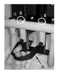
Separate the two halves of the black strap and bring towards the front.
