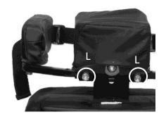
Loosen the bolt (L) securing the lateral support. Adjust to the desired location and tighten the bolt. Ensure they are symmetrical and centrally aligned.
