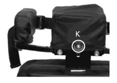
These two components adjust together. Loosen the single bolt (K) securing the assembly and move the supports to the desired location. Tighten the bolt. Check the Hip to Axilla height to ensure it ties in with the Heel to Axilla measurement.
