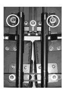
Loosen the top bolts of both the Thigh Supports (I). Adjust the height to the desired location. Retighten the bolts.
