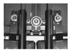
To adjust the secondary adjustment, loosen the bolt (E) at the centre of the Body Support that runs in the adjustment slot. Lift or lower the Body Support to the correct height. Tighten the bolt fully.
