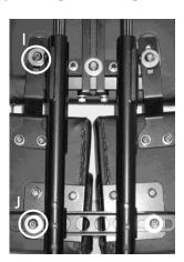
Loosen the top (I) and bottom (J) bolts of the Thigh Support that you want to adjust (work with one side at a time to ensure both thigh supports remain at the same height). Adjust the support to provide that appropriate amount of ab/adduction. Tighten the bolts. Adjust the other Thigh Support if necessary in the same way.
