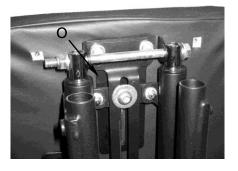
Once they have been removed, rotate the plate through 180° (O) and insert back onto the Body Support (this ensures the correct spacing of the sliding mechanism is retained).
