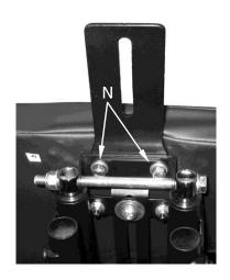
Carefully loosen and remove the two 10mm bolts (N) securing the Chest Support Vertical Adjustment plate.
